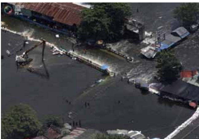
A levee breach leading to flooding
