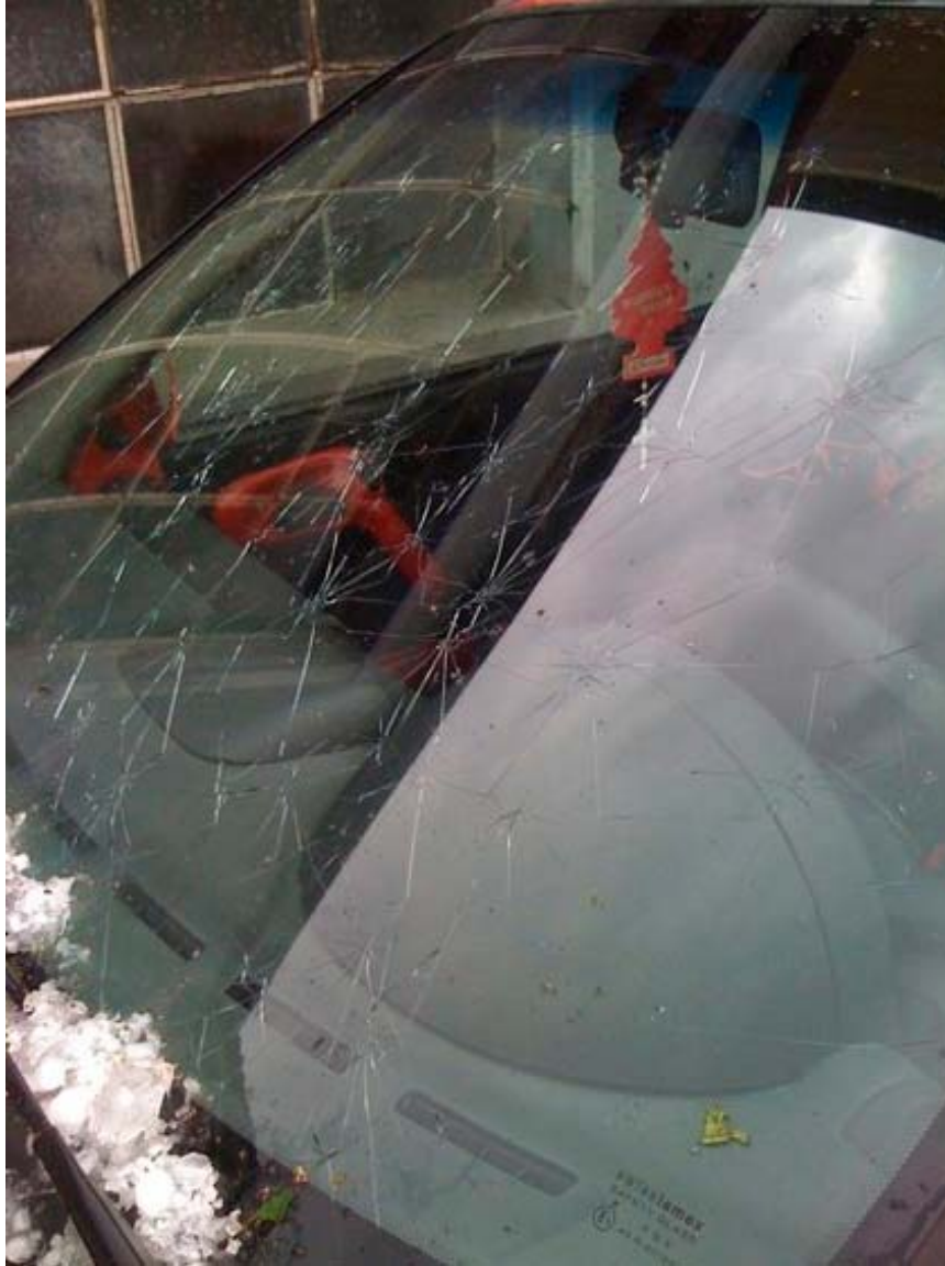
Figure 10: Example of car windscreen damage
